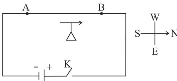
(i) In which direction will the needle deflect when the key is closed?
